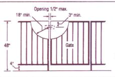
Use this as a guide when the release mechanism is located less than 54 inches
